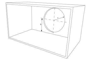
Figure 1. Measurements for cutting hole in panel
