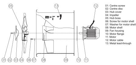
Figure 5. Exploded drawing of ACL fan
