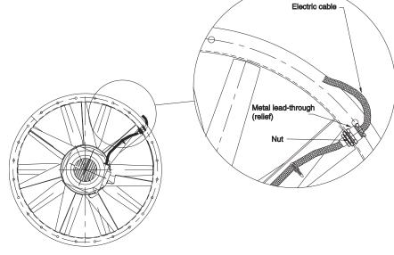
Figure 6. Electrical connection through fan housing
